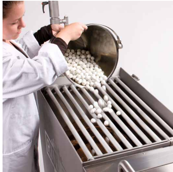
Protective grid: with automatic safety device. Heatable mass container: mass remains temperature-constant.
