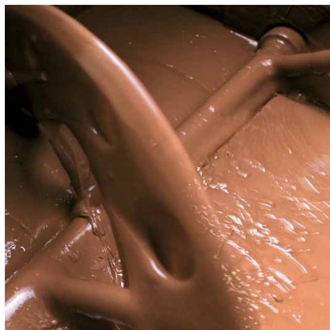
Horizontal stirrer: keeps mass homogenous – even with extremely light added ingredients.
